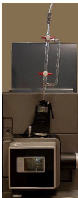
Figure 1. Waters Xevo QTof mass spectrometer fitted with a vertical loading ASAP inlet port with a glass sample delivery probe in position.
