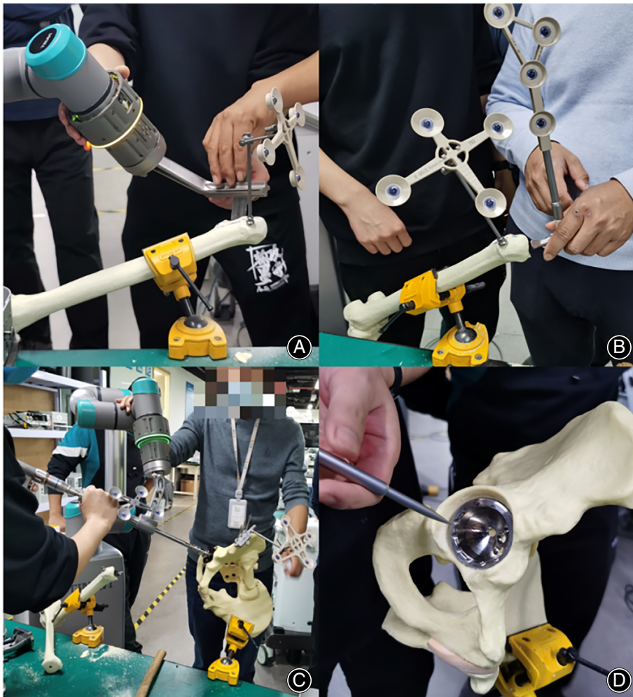
FIGURE 12 RA group operation process (A) Robot-assisted femoral neck osteotomy; (B) Femoral anteversion measurement; (C) Robot-assisted acetabular grinding; (D) Cup parameters verification
