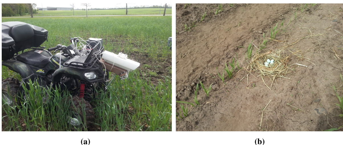
Figure 1. Photos from data collection. (a) Thermo-visual setup mounted on an all-terrain vehicle; (b) man-made skylark nest with heated plastic eggs.
