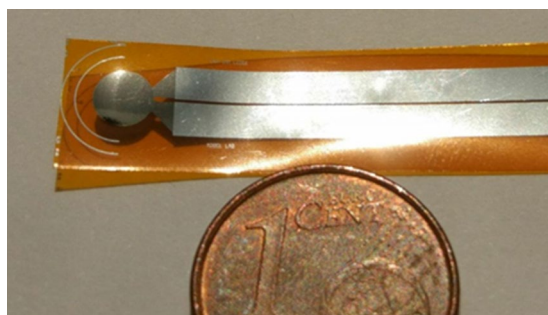
Figure 6. Image of the realized pressure sensor on Kapton substrate.
