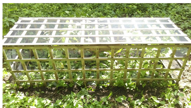
Figure 8. A snail cage made of wooden slats covered with a dense mesh net used in the experiment. The mesh size is ca. 1.5 mm to prevent snails escape.
