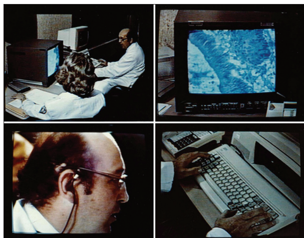
Figure 8: Live demonstration (in 1986) of the first operational robotic telemicroscopy system in history. Top left: Dr. Alexander Miller and associate operating the robotic telemicroscopy system; top right: example of the video feed from the system; bottom left: Close-up of videoconferencing gear worn by participants; bottom right: Close-up demonstrating keyboard control of remote robotic microscope
