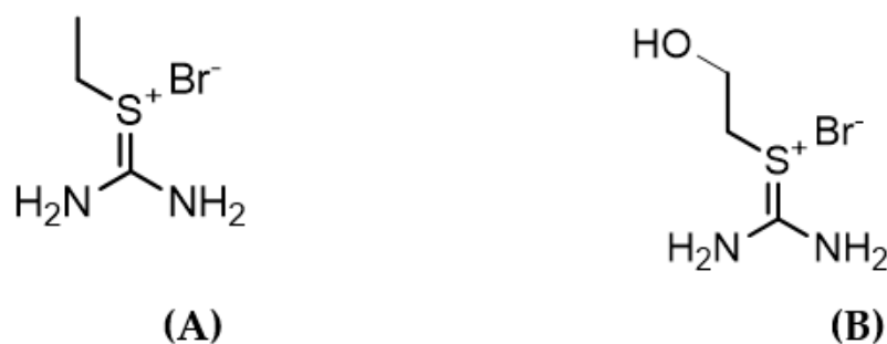
Figure 1. Structures of the ionic liquids used in this work. (A) 2-ethylthiuronium bromide and (B) 2-(hydroxyethyl)thiuronium bromide.
