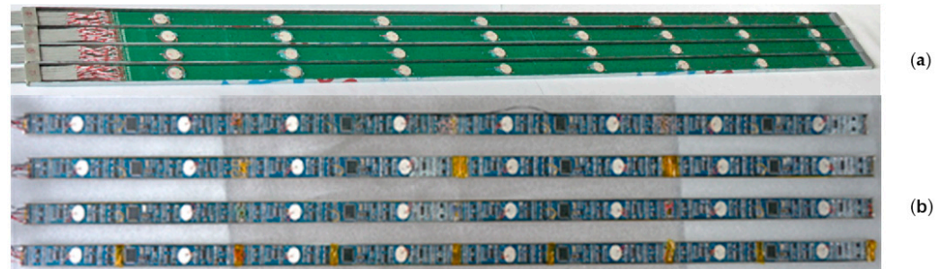
Figure 12. Traditional reception circuits (a), and intellectualized active reception circuits (b).
