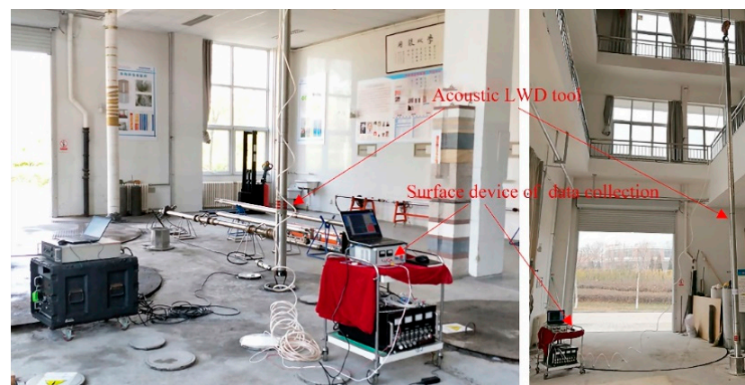
Figure 15. Acoustic LWD testing in room well group.
