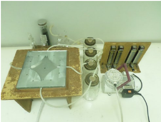
Figure 1. Four-arm olfactometer device used for the different tests. Picture: Apolline Sanou.
