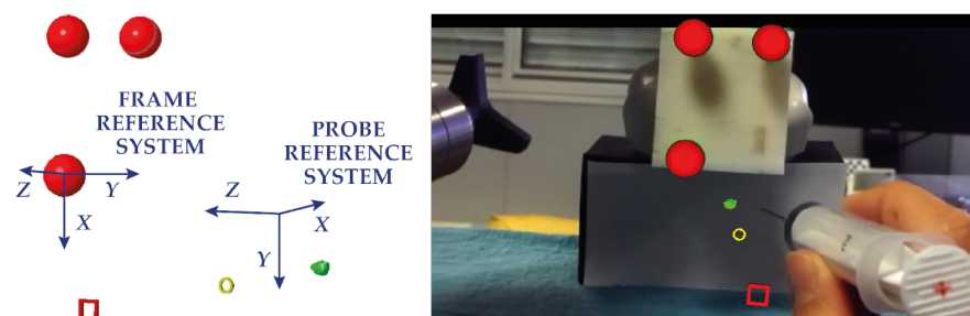
Figure 10. Augmentation of the real scene. On the (left), the 3D CAD modelling of the virtual elements used to augment the real scene. On the (right), the AR image visualized through the HMD.
