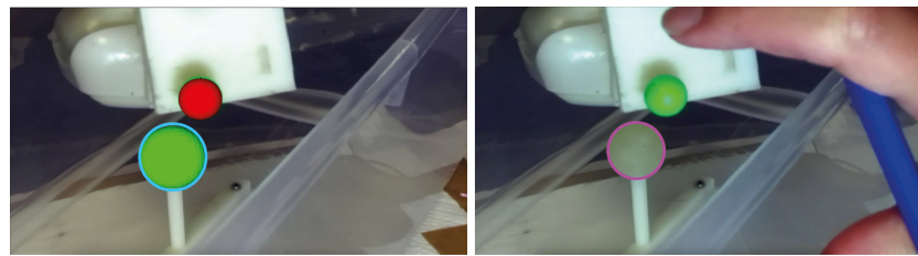
Figure 7. Example of image processing for detecting real and virtual spheres. On the (left), the AR image: the real scene is augmented with the virtual sphere (in green) registered over the lollipop's head and the tracked optical frame (in red). The detected virtual sphere is represented by a blue circle. On the (right), the real image: the detected real lollipop's head is represented by a magenta circle.
