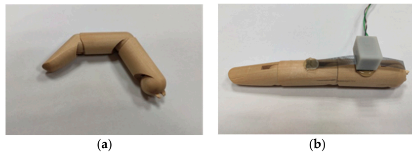
Figure 10. Response testing device. (a) Wooden finger; (b) Wooden finger with a sensing unit.
