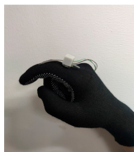
Figure 12. The designed glove with a sensing unit on it.
