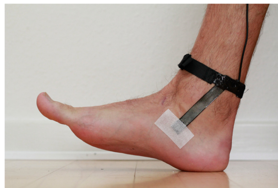
Figure 1 The stretch-sensor is attached on the medial side of the foot between 20 mm posterior to the malleolus medialis, and 20 mm posterior to the navicular tuberosity.
