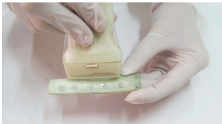
FIGURE 5: Ultrasonic gel was applied on the intact surface on the linear ultrasonic probe that was placed on the block.
