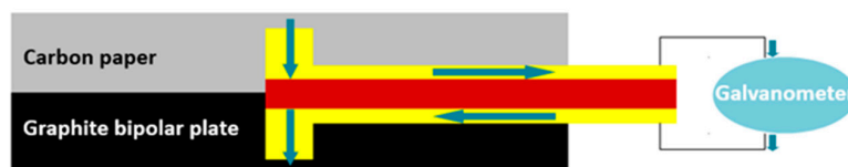
Figure 3. Schematic diagram of the principle of the micro current sensor.
