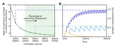
**Fig 4. Summed conductance of feedback NMDAR synapses as a function of frequency.** (A) Spike trains of different frequencies were delivered to a model NMDAR synapse with a closing time of 80 ms, and the maximum conductance recorded experimentally. (B) Faster spike trains produced a larger maximum conductance. At the frequencies of tadpole swimming, the conductances did not rise above ~3 times the conductance of a single NMDAR synaptic event (yellow trace).
