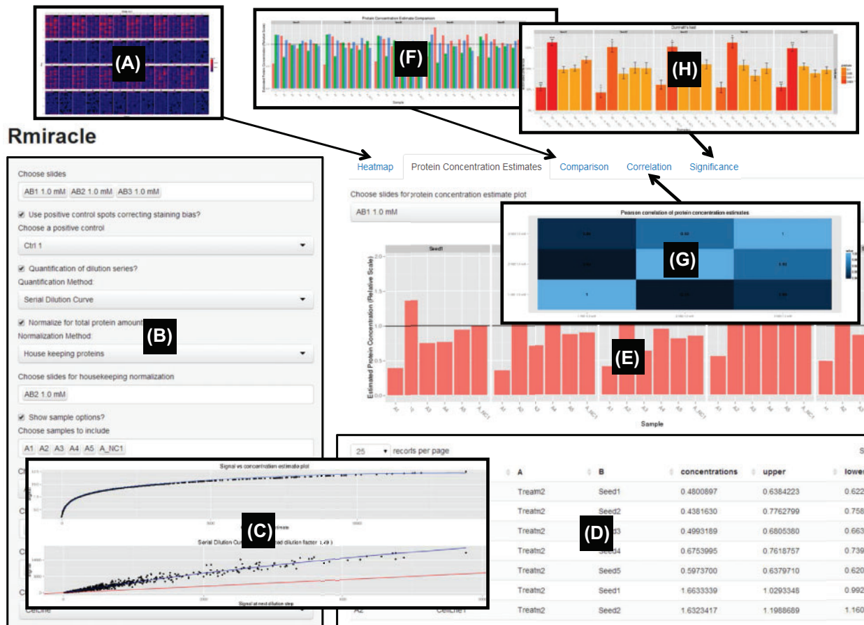
Fig. 5. Analysis using Rmiracle: A heatmap visualizes different slide properties, such as signal intensities (A). Users can change various parameters, for example inclusion of surface adjustment, selection of methods for quantification and normalization for total protein amounts. Specific samples can be selected and grouped based on different properties of the data set (B). Depending on the quantification method, diagnostic plots are shown (C). The results are displayed in an interactive table and in a bar plot (D and E). A global overview of protein concentration estimates is available for all slides and plate-based readouts (F). Pearson correlation coefficients are calculated for all slides, as well as for plate-based readouts (G). Significance is assessed by comparing sample groups to negative controls through Dunnett's test (H)
