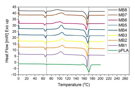
Figure 8. DSC heating scans of melt-blown nonwovens.
