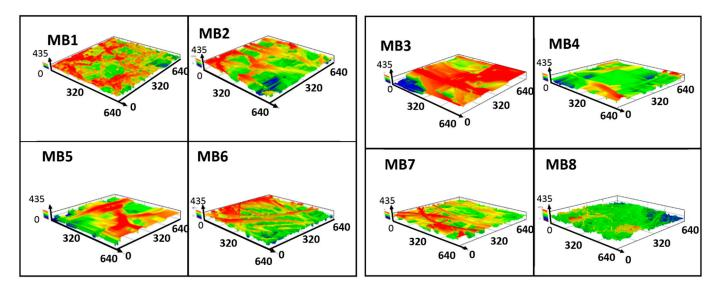
Figure 5. PLA nonwovens surface profile of the rough surface found in 3D laser microscopy.
