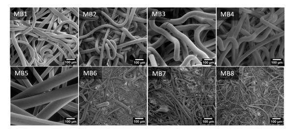
Figure 2. Scanning electron microscopy photography of nonwoven scaffold MB1-8.
