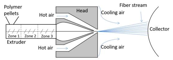
**Figure 1.** Meltblowing process diagram with the extruder and its zones: zone 1—the feed zone; zone 2—the transition zone; and zone 3—the metering.
