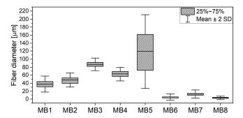
Figure 3. Fiber diameter distribution of PLA melt-blown scaffolds.
