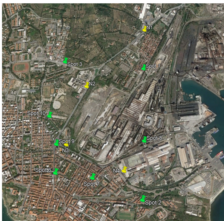
Figure 8. Aerial picture of Piombino with the positioning of long term (yellow) and short term (green) measurements. “Spot” measurements are the short-terms one, while the “N”s are the long-term.
