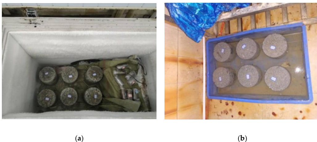
Figure 6. Freeze–thaw cycle and water-stability test: (a) freeze–thaw test; (b) water immersion.
