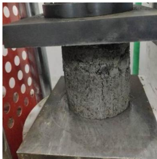
Figure 2. Axial compressive-strength test.
