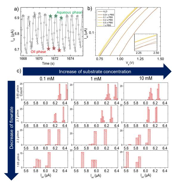
**Figure 3.** FET response to variations in sample composition. (a)  $I_{sd}$  signal change with passing droplets. Local maxima correspond to every single droplet, while minima correspond to the oil separating them. (b) Transfer characteristics response to phosphate-buffered saline (PBS) buffer ionic strength variations. The calibration of the flow-rate test is shown in (c).
