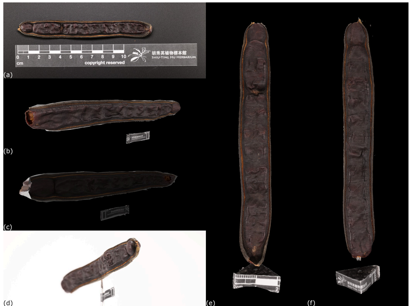
Fig 6. Comparison of 3D models of long dimension carpological material reconstructed by different positioning. (a) A carpological material of the fruit of Samanea saman (Jacquin) Merrill J. Wash (PH044). (b)&(c) The 3D model when PH044 was placed horizontally. The structure on the front side was reconstructed but the back side was not, as shown by the regions with darker color. (d) Decrease in sharpness of the images of PH044 was found due to greater depth of field from two ends, which reduced the coherence between images so the software could not recognize its structure for further reconstruction. (e)&(f) The 3D model when PH044 was placed vertically. The structure was reconstructed completely on both sides.
