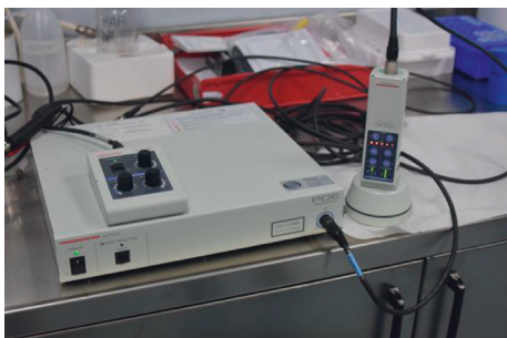
FIGURE 10: PDE probe (PhotoDynamicEye Hamamatsu by SEDA S.P.A. Italy) handheld fluorescence imager.
