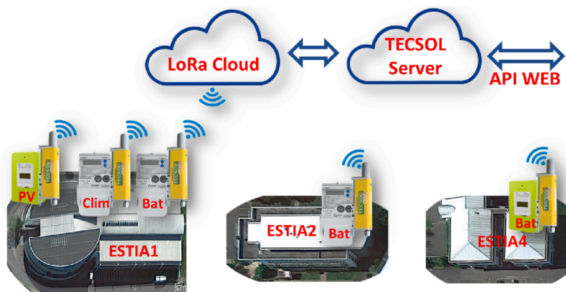
Fig. 3. Tecsol TICs connected to the meters in the three buildings.
