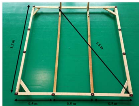
Figure 3. Schematic representation of the custom cart built for tags accommodation and predetermined distances between tags.
