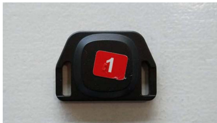
Figure 2. Tags use Bluetooth Low Energy to send a radio signal to a positioning engine, which uses proprietary algorithms to calculate the tag position ( 44 \times 31 \times 8 mm, 10 g).
