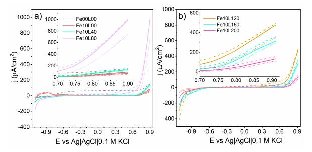
**Figure 10.** Records of linear voltammetry carried out in darkness (dotted), under simulated solar (dashed), and visible (solid) light for (**a**) bare titania and with Fe film further treated with 40 and 80 mJ/cm<sup>2</sup> and (**b**) 120,160, and 200 mJ/cm<sup>2</sup>.
