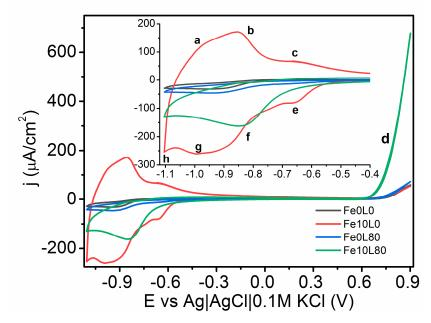
**Figure 9.** Cyclic voltammetry recorded for pristine and laser-modified; (80 mJ/cm<sup>2</sup>) TiO<sub>2</sub>-NTs in 0.5 M NaOH electrolyte in darkness.
