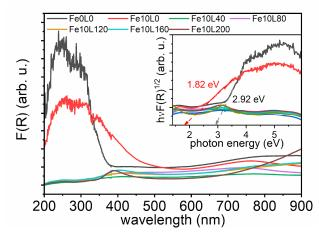
Figure 8. Absorbance spectra and Tauc plots (inset) for laser-treated Fe-decorated TiO<sub>2</sub>-NTs.
