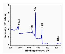
Figure 6. The XPS survey spectrum recorded for Fe10L80 sample.
