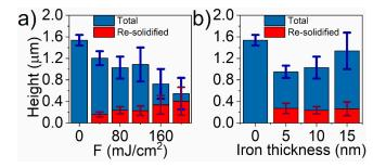
**Figure 3.** The dependence of the length of titania nanotubes (**a**) with 10 nm deposited Fe on the applied laser fluence and (**b**) on the iron layer thickness when the applied laser fluence equals 80 mJ/cm<sup>2</sup>.
