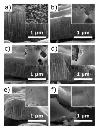
**Figure 2.** SEM images of laser-treated titania nanotubes (TiO<sub>2</sub>-NTs) covered by 10 nm Fe film from top (inset) and side. Images show the samples (**a**) untreated and treated by laser of (**b**) 40 mJ/cm<sup>2</sup>, (**c**) 80 mJ/cm<sup>2</sup>, (**d**) 120 mJ/cm<sup>2</sup>, (**e**) 160 mJ/cm<sup>2</sup>, and (**f**) 200 mJ/cm<sup>2</sup> fluence.
