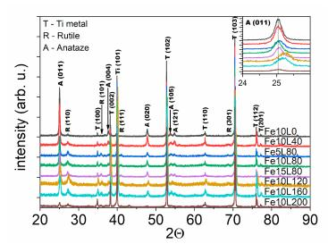
Figure 4. X-ray diffraction patterns of laser-annealed Fe-decorated TiO<sub>2</sub>-NTs.
