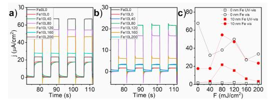
**Figure 11.** Transient photocurrents recorded for the bare and laser-annealed Fe-decorated  $TiO_2$ -NTs in 0.5 M NaOH electrolyte under the light of full solar (**a**) and limited to visible (**b**) spectrum. Light-on current plateau of chronoamperometry records in UV-vis (circle) and visible light (square) are shown in graph (**c**).
