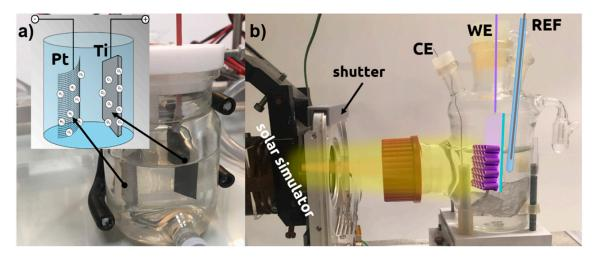
**Figure 1.** The experimental setups used for (**a**) the anodization and (**b**) photoelectrochemical characterization.
