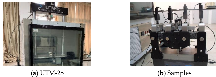
Figure 4. Four-point bending fatigue test.
