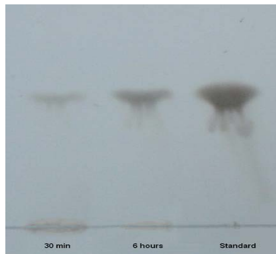
Figure 6. Thin layer chromatography of the reaction products of polygalacturonic acid hydrolyzed by PG. Hydrolysis times were 30 min and 6 h. Standard was 10 g/L of monogalacturonic acid.
