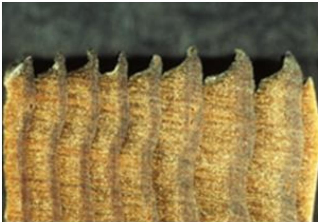
**Figure 9.** Rough surface of wood after weathering.
