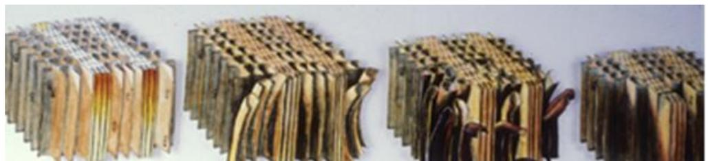
**Figure 7.** Loss of surface fibers due to UV degradation of lignin.
