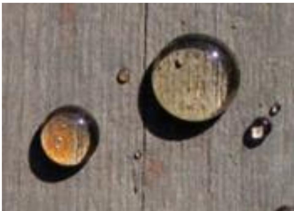
**Figure 19.** Water droplets on wood with a nanozinc oxide coating.
