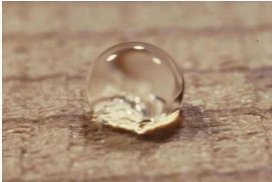
**Figure 5.** Water droplet on the surface of water repellent treated wood.
