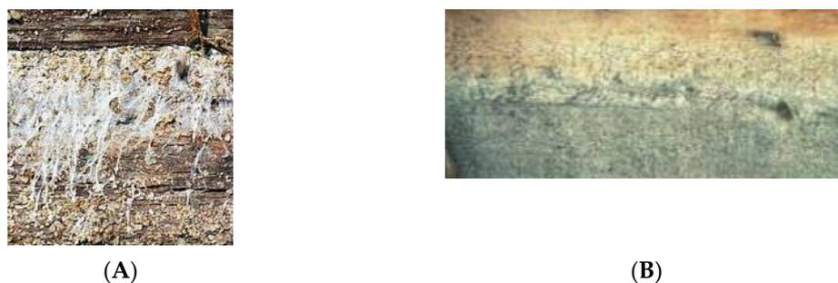
**Figure 21.** White rot fungi growing on a wood surface (A) and mold growing on a painted wood surface (B).
