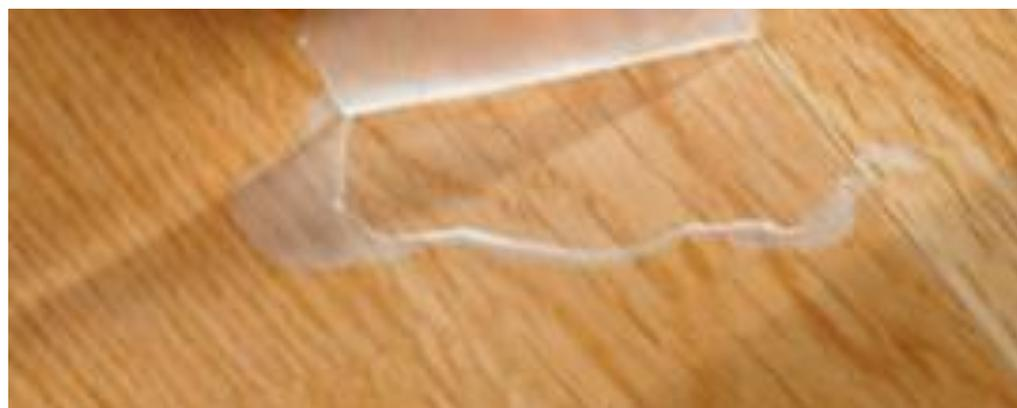
**Figure 18.** Clear coating failure.
