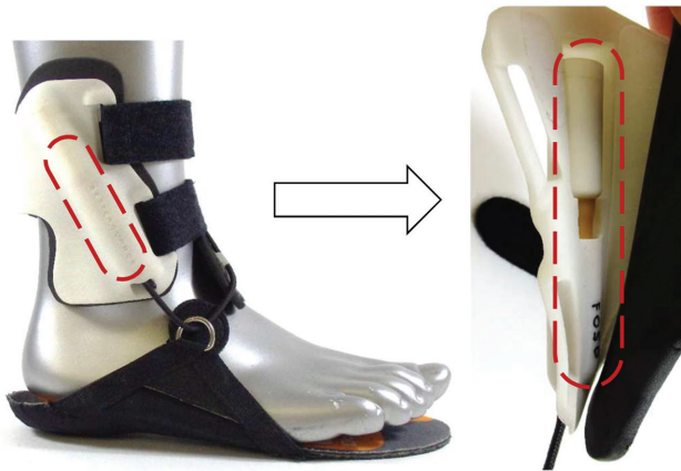
Figure 1. Depiction of the external ankle brace used for testing (left), with the exchangeable module indicated by the dashed line, which is visible only upon lifting the cushioning pads (right). The brace was designed to ensure that participants and investigators were blinded to the module used (active or passive).
