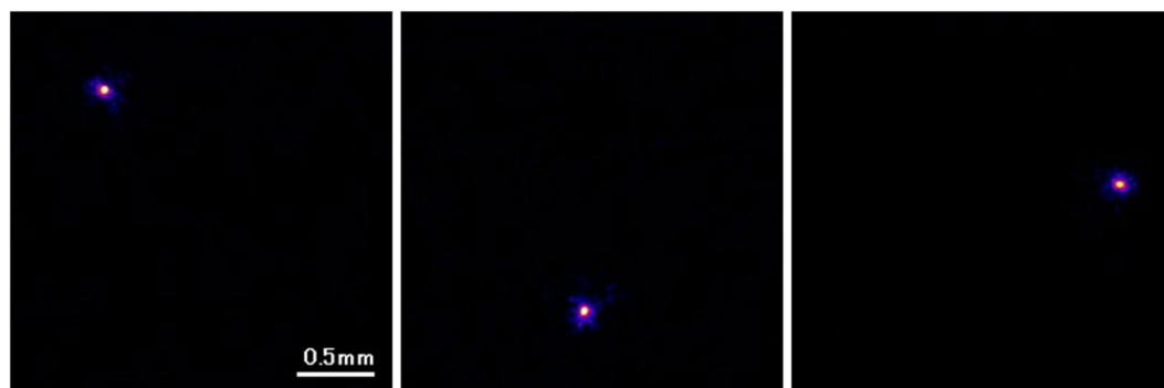
Figure 6. Images of typical alpha particles measured by developed imaging system.
