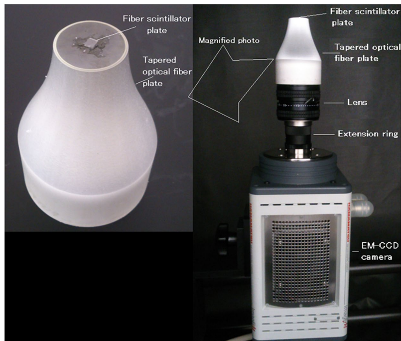
Figure 4. Developed ultrahigh resolution radiation imaging system; right side photo shows whole system and left side is its upper part.
