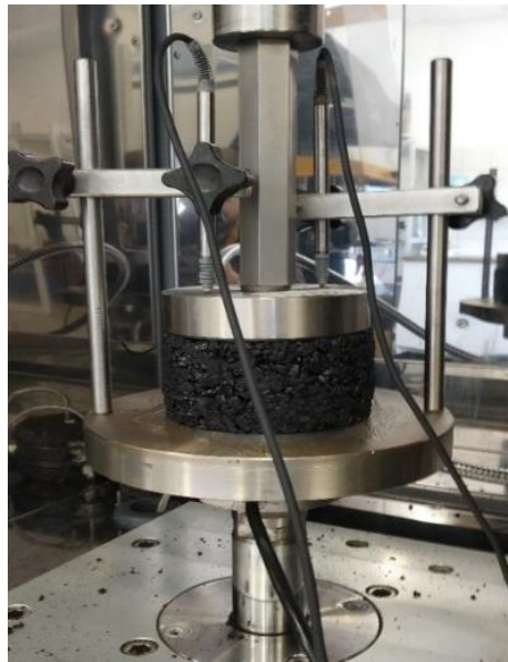
Figure 2. Test stand for the determination of uniaxial cyclic compression.
