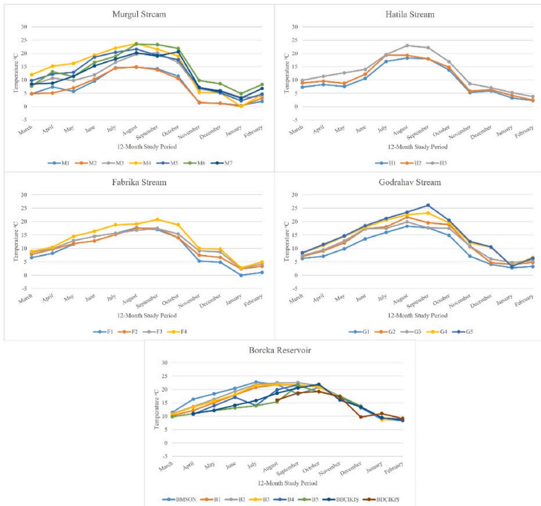
Fig. 8. Annual water temperature changes for the streams of Murgul, Hatila, Fabrika, and Godrahav and for the reservoir of Borcka Reservoir.
