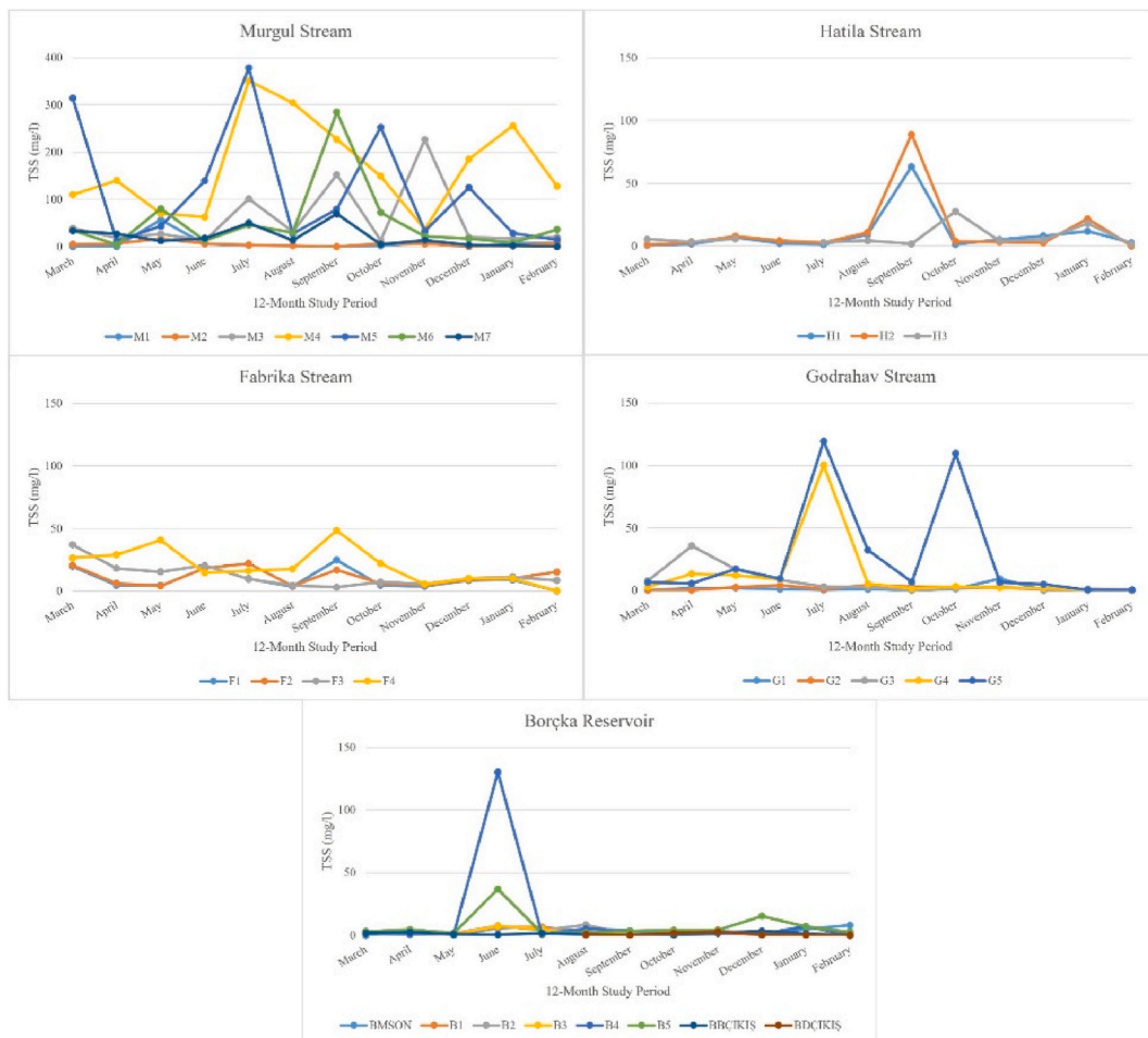
Fig. 15. Monthly changes of TSS for the streams of Murgul, Hatila, Fabrika, and Godrahav and the reservoir of Borçka Dam.
