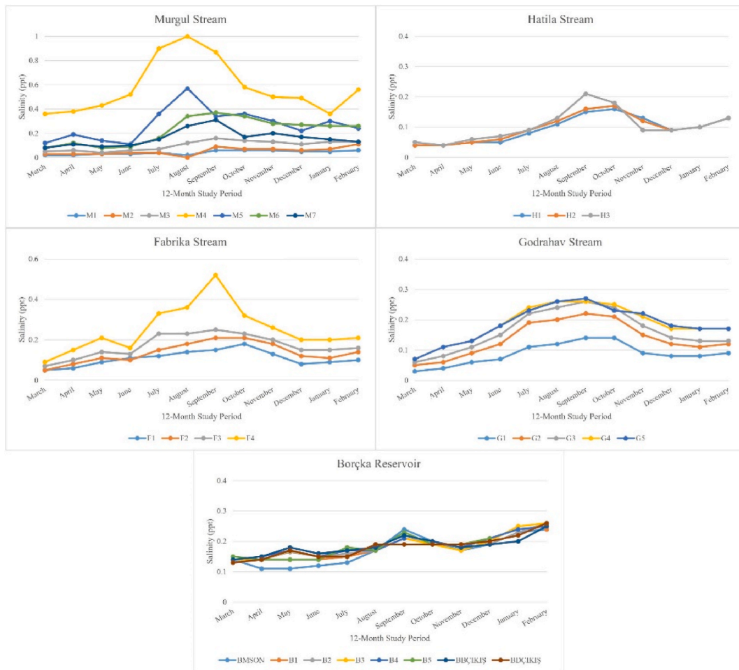
Fig. 11. Monthly changes of salinity values for the streams of Murgul, Hatila, Fabrika, and Godrahav and the reservoir of Borcka Dam.
