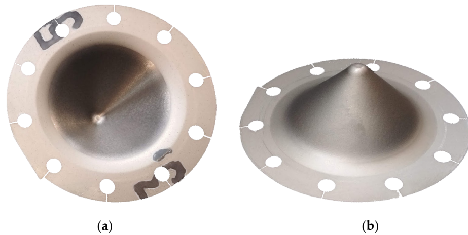
Figure 4. Successfully formed specimen: (a) inner side (b) outer side.
