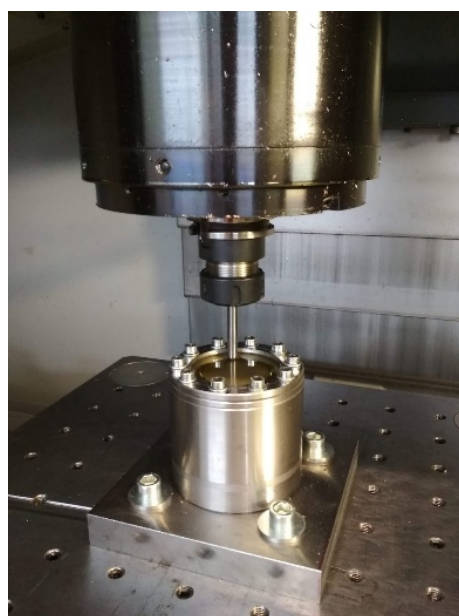
Figure 1. Forming device mounted inside CNC milling machine workspace.
