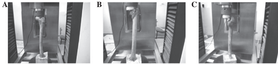
Figure 1. Load relaxation experiment images of the specimens in three groups. (A) Load relaxation experiment image of the control. (B) Load relaxation experiment image of the traditional type of prosthesis implantation group. (C) Load relaxation experiment image of the preservation of femoral neck prosthesis implantation group.
