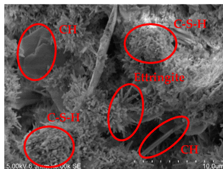
Figure 8. SEM image at 5000× of B24R16 specimen.
