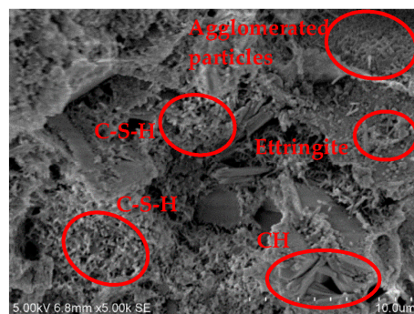
Figure 7. SEM image at 5000× of B36R4 specimen.
