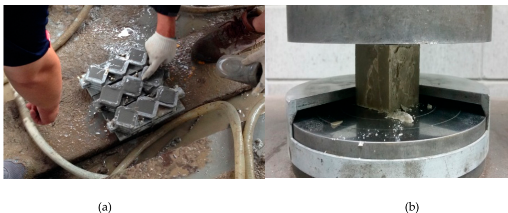
Figure 4. Test methods of homogel strength: (a) Molding of cubic molds for homogel strength test; (b) homogel strength test.
