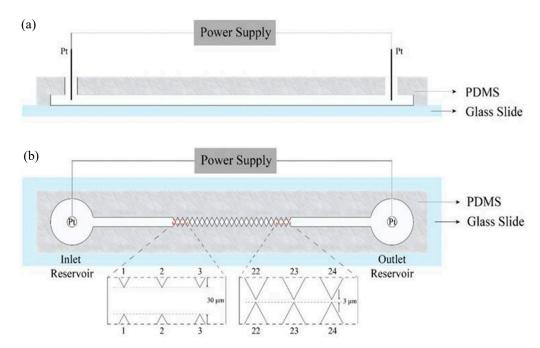
**Figure 4.** Illustration of the sawtooth g-iDEP device. (a) side view and (b) top/vertical view. From saw tooth gates 1 to 24, the channel is constricted to an increasing degree by triangular insulting wall protrusions. These constricted zones and structures act as capturing zones due to local increases in electric fields and gradients [103]. ©Figure 4 reproduced with Copywrite clearance and reprinted (adapted) with permission from: Copywrite (1876) Royal Society of Chemistry ID 1044809-1.
