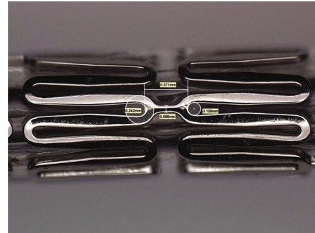
FIGURE 2: Envision stent, 3.5 \times 28 (crimped).
