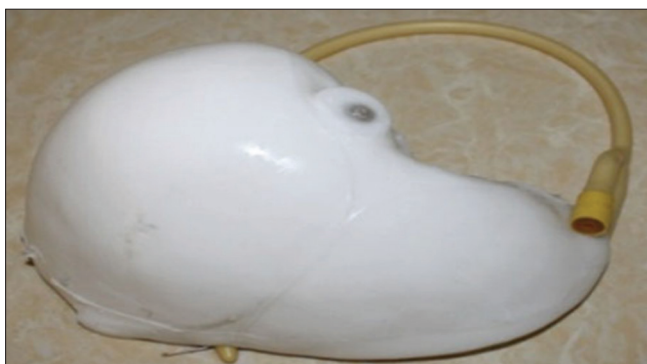
Figure 2: Polyvinyl alcohol cryogel-liver phantom [15]
