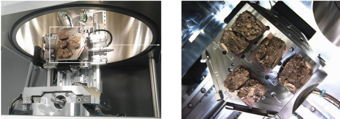
**Figure 3.** A small portion of the specimens placed onto the Apreo SEM scanning table.
