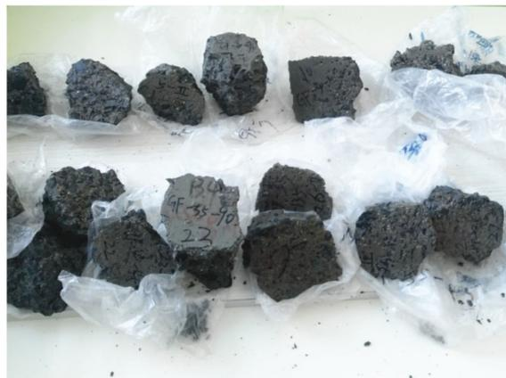
**Figure 2.** A portion of the blocks after freeze-thaw cycles.
