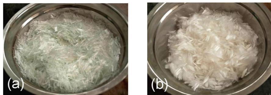
**Figure 1.** Appearance of the used fibers: (a) GF and (b) PPF.**Table 6.** Properties of GF and PPF.
