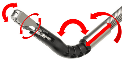
Figure 2. Movements of the articulating arm and rotatable grasper: gripping and rotation of the grasper, flexion, rotation, and advancement of the articulating arm.
