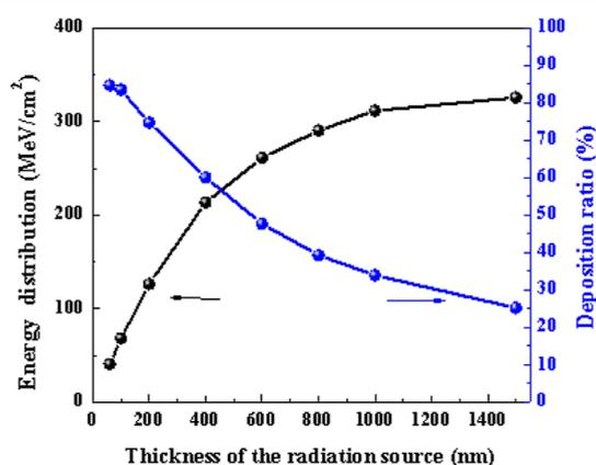
**Figure 6.** Energy deposition and deposition ratio of incident particles with different radiation source thicknesses based on  $Ti^3H$ .
