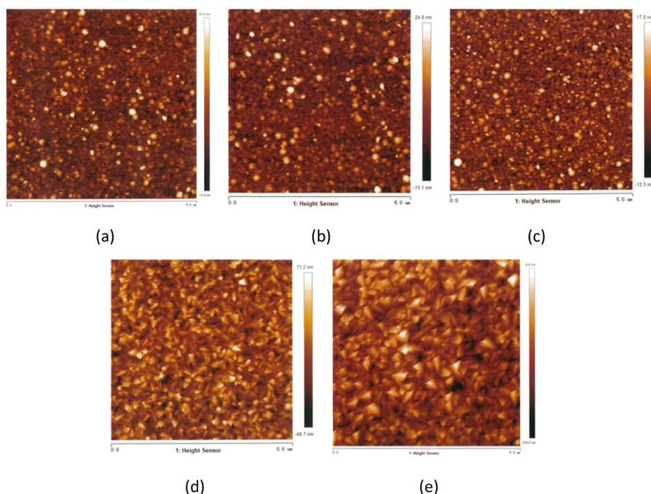
**Figure 2. Height maps of titanium films obtained with different sputtering parameters: (a) sample no. 1; (b) sample no. 2; (c) sample no. 3; (d) sample no. 4; and (e) sample no. 5.**
