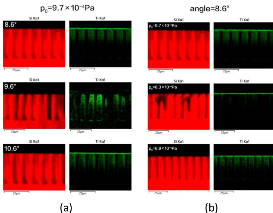
**Figure 4.** EDS surface scanning results of titanium coating under different initial conditions: (a)  $p_0 = 9.7 \times 10^{-4}$  Pa with different coating angles and (b) coating angle =  $8.6^\circ$  with different background pressures.
