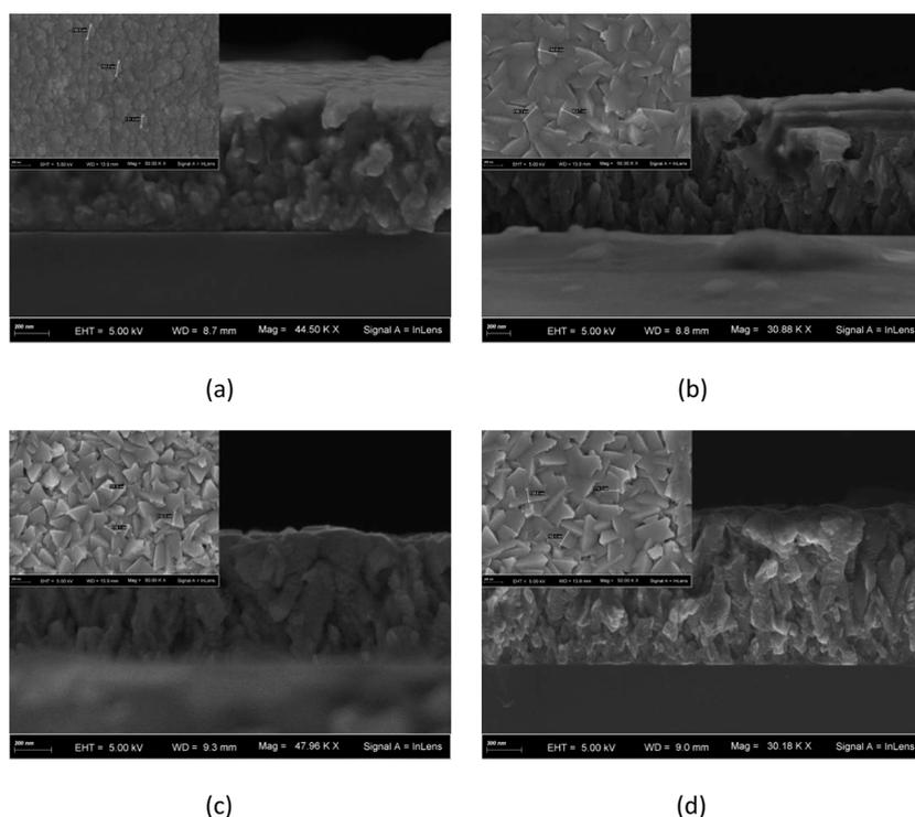
**Figure 3.** SEM images of the surface and cross-section of titanium thin films obtained with different sputtering parameters: (a) sample no. 4; (b) sample no. 6; (c) sample no. 7; and (d) sample no. 9.
