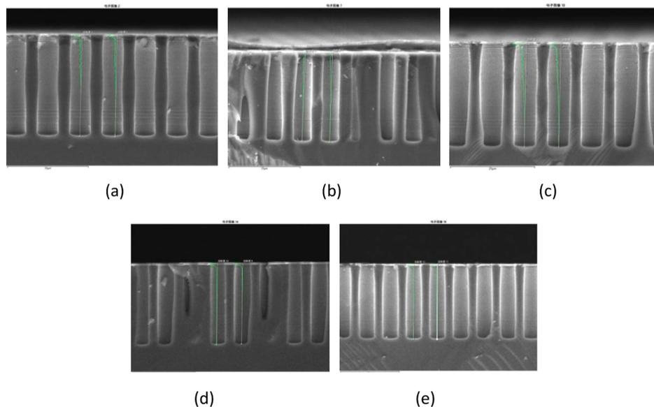
**Figure 5.** EDS line scan results of titanium coating under different initial conditions (figures a–e show samples TD-1, TD-2, TD-3, TD-4, and TD-7 in sequence).
