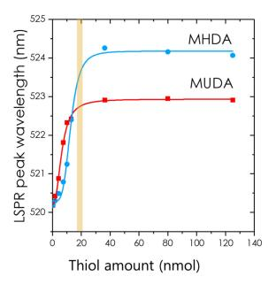
**Figure 4.** Evolution of the LSPR peak wavelength as a function of the added amount of thiol molecules in the case of MUDA (red square) and MHDA (blue circle). The curves are guides for the eye. The wide vertical line represents the transition threshold to the plateau and indicates that the full coverage of the nanoparticle is reached.
