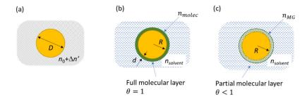
**Figure 6.** (a) A spherical nanoparticle of diameter D in a medium of index  $n_0 + \Delta n'$  (b) nanoparticle functionalized by a molecular layer of thickness d, in a medium of index  $n_{solvent}$ , (c) the same nanoparticle with a partial coverage  $\theta < 1$ . The refractive index of this partial monolayer  $n_{MG}$  is calculated with the Maxwell–Garnett formula.
