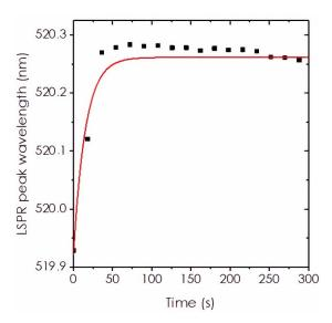
Figure 5. Evolution of the LSPR peak wavelength with time, providing information on the kinetics of functionalization of AuNPs with MUDA. Solution was not stirred during the acquisition. First, 50  $\mu$ L of MUDA at 35  $\mu$ M was added to 2 mL of AuNPs at 0.66  $\times$  10<sup>-9</sup> mol/L, leading to a final MUDA concentration of 0.86  $\mu$ M in the reacting solution. The red line corresponds to a fit of the data with a single exponential.
