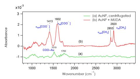
**Figure 2.** FTIR (Fourier Transform Infra-Red) absorption spectra of two AuNPs solutions, centrifugated and dropcasted on a silicon substrate, recorded in transmission with 70° incidence. Spectrum (a) corresponds to the Turkevich solution after centrifugation and spectrum (b) corresponds to the AuNP solution after functionalization with MUDA.
