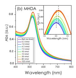
**Figure 3.** UV-visible spectra in solution of the progressive adsorption of (**a**) MUDA and (**b**) MHDA on 22 nm gold nanoparticles. The LSPR shift is 2.7 nm and 3.9 nm for MUDA and MHDA, respectively (see text for discussion). The insets show a zoom-in of the LSPR peak maximum.
