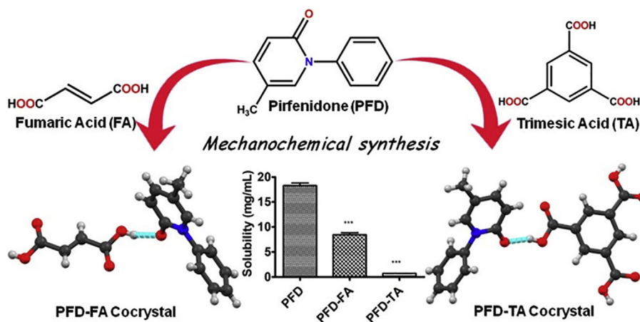
Figure 22 Chemical structure of pirfenidone (PFD), fumaric acid (FA) and trimesic acid (TA); hydrogen bonding between the PED–FA cocrystal and PFD–TA cocrystal; solubility results of the PFD, PFD–FA and PFD–TA cocrystals. Adapted from the Ref. 175 with the permission. Copyright © 2019 American Chemical Society.
