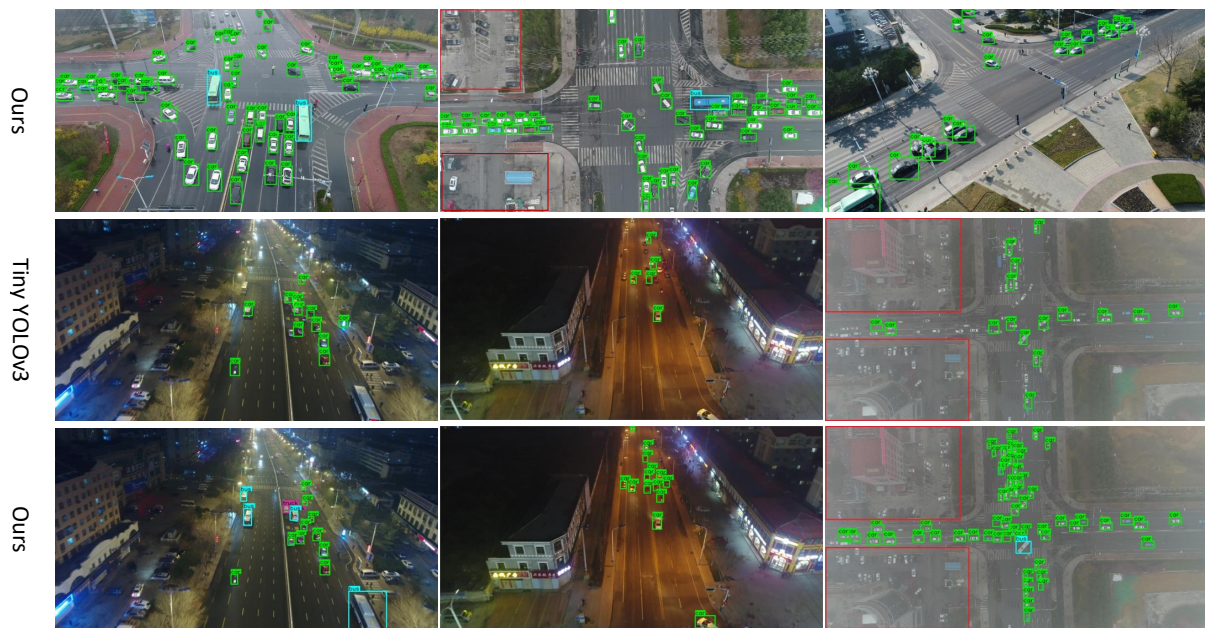
Figure 4. Some visualization results of our proposed method and Tiny YOLOv3. The first two lines of images are from the validation set of Visdrone-2018-VID; the last four lines of images are from the testing set of UAVDT-DET. In each comparative example, the top picture shows the results of our method, the bottom picture shows the results of Tiny YOLOv3. The areas inside the red rectangles have no annotations, so we did not detect these areas.
