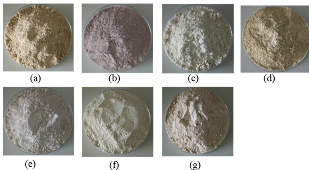
Figure 2. Clay samples showing colour variations: (a) Afuze (orange-brown), (b) Ihitte (pink), (c) Kutigi (white), (d) Minna (orange-yellow), (e) Nsu (light brown), (f) Oboro (grey-white) and (g) Obowo (yellow- brown).
