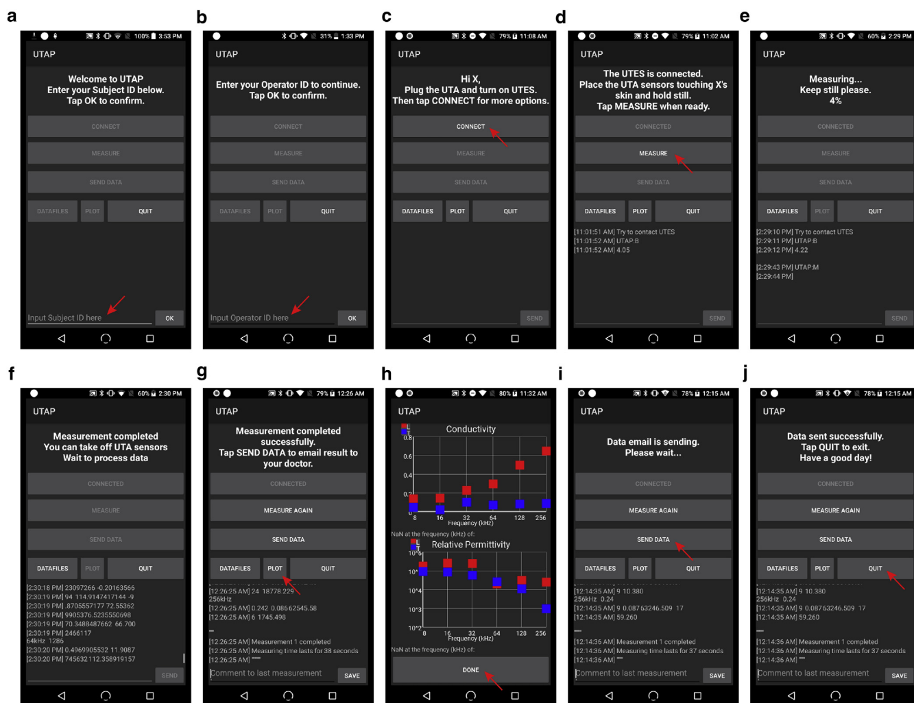
Supplementary Figure S1. Application–user interface. The application guides the operator from step a to j to complete measurement and e-mail the data for further analysis.
