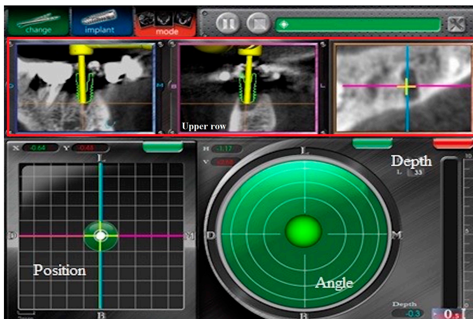
Figure 2. The monitor shows the depth, position, and angle of dental implant. The upper row shows the real-time labial view, sagittal view, and occlusal view (upper row from left to right). This figure was authorized by Taiwan Implant Technology Company.
