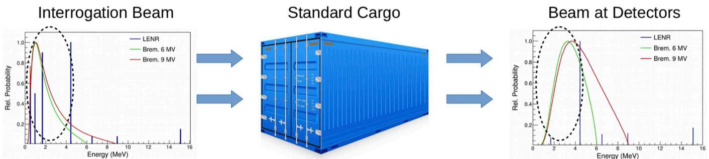
Fig 1. Work-flow of a cargo scanning system from a radiation detection standpoint. The left shows the energy distribution of various interrogation beams and the right shows the energy distribution of those beams after penetration through the container. The black circle highlights the differences in the low-energy end of the spectrum.
