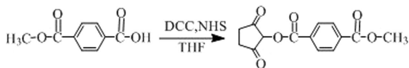
Figure 2. The synthesis illustration of terephthalic acid methyl ONSu ester.
